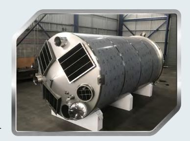
ensuring quality and compliance. Our focus on hygienic vessels for the food and beverage industry is evident in our range, which includes milk silos, cream tanks, yoghurt processing vessels, lauter tuns, fermenters and milk powder bins.
